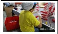
NC photo 1: 2 out of 4 cleanser using workers in the packing workshop on the 3F of the production building wore the cotton gloves instead of the rubber gloves, and did not wear the active carbon masks in work.
