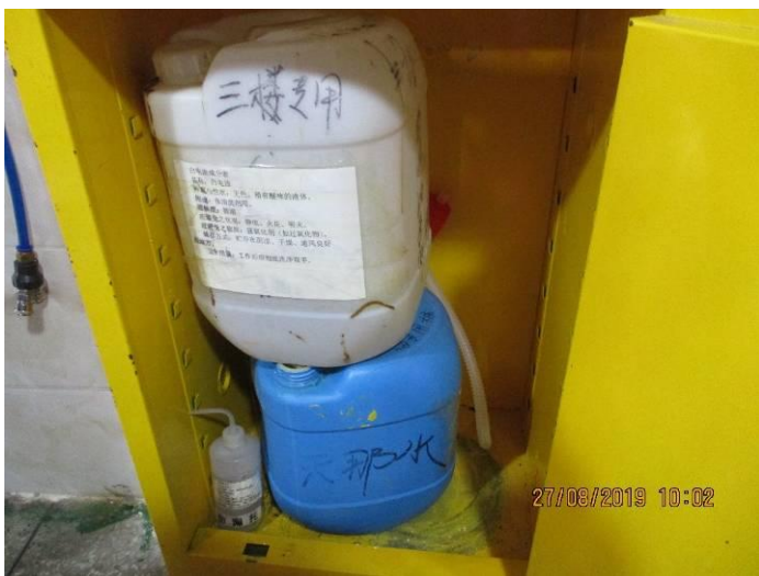
Chemicals stored with secondary containment
